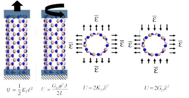
Fig. 3: Boundary conditions imposed on BNNTs: (a) Tensile, (b) Twisting, (c) In-plane biaxial tension, and (d) In-plane shear
