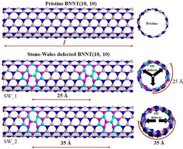
Fig. 2: Schematics representation of pristine and SW defected (10, 10) BNNT
