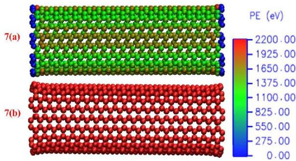
Fig. 7: Failure of BNNTs under in-plane bi-axial tension
