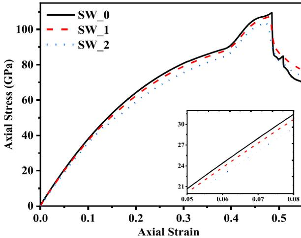
Fig. 4: Stress-strain curves for (10, 10) BNNTs
