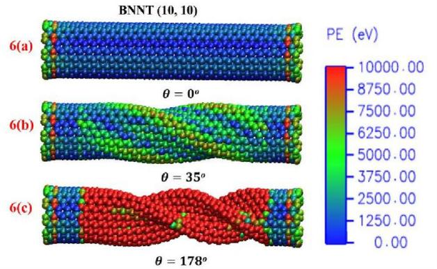
Fig. 6: Snapshot of twisting of pristine armchair (10, 10) BNNT.
